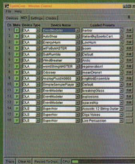
The mission control editor enables sound designers to combine as many as 16 DLAs simultaneously
